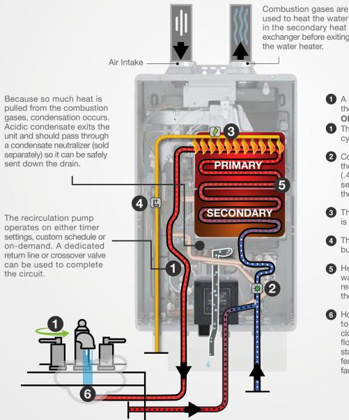
used to heat the water in the secondary heat exchanger before exiting the water heater.
